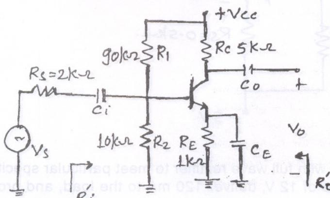
4. (a) In a germanium transistor using potential divider biasing method, the operating point is chosen such that  $I_C = 2\text{mA}$ ,  $V_{CE} = 4\text{V}$ . If  $R_C = 2\text{k}\Omega$ ,  $V_{CC} = 10\text{V}$ , and  $\beta = 50$ . Determine the values of  $R_1$ ,  $R_2$ , and  $R_E$ . Assume  $I_I = 10 I_B$ .  $I_I$  is current through  $R_1$ .
