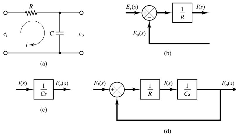
A complicated block diagram involving many feedback loops can be simplified by a step-by-step rearrangement. Simplification of the block diagram by rearrangements considerably reduces the labor needed for subsequent mathematical analysis. It should be noted, however, that as the block diagram is simplified, the transfer functions in new blocks become more complex because new poles and new zeros are generated.
