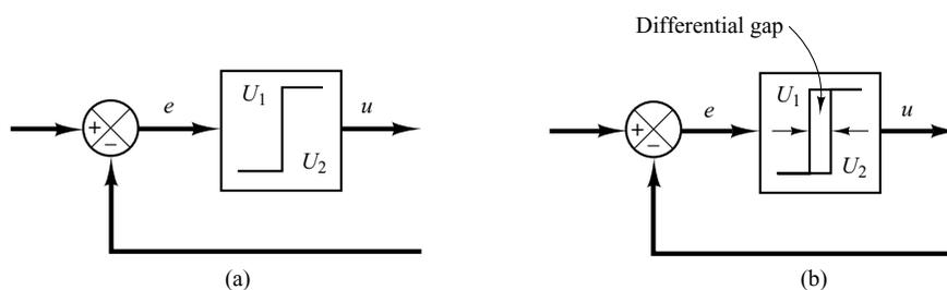
is called the *differential gap*. A differential gap is indicated in Figure 2-7(b). Such a differential gap causes the controller output  $u(t)$  to maintain its present value until the actuating error signal has moved slightly beyond the zero value. In some cases, the differential gap is a result of unintentional friction and lost motion; however, quite often it is intentionally provided in order to prevent too-frequent operation of the on-off mechanism.
