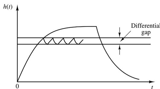
From Figure 2–9, we notice that the amplitude of the output oscillation can be reduced by decreasing the differential gap. The decrease in the differential gap, however, increases the number of on–off switchings per minute and reduces the useful life of the component. The magnitude of the differential gap must be determined from such considerations as the accuracy required and the life of the component.
