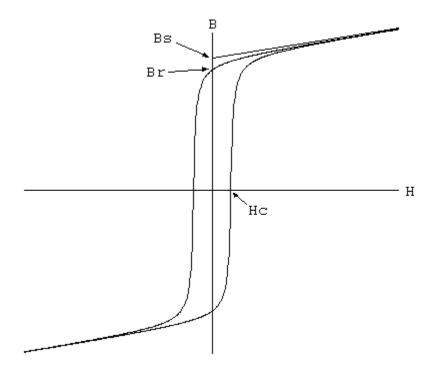
The initial magnetization curve is given by
