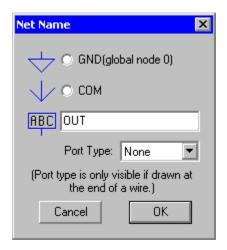
It is possible to indicate that a node is a port of type input, output, or bi-directional. These port types will be drawn differently but have no significance to the netlister. Indicating a port type can make circuit more readable. Global nodes are also drawn differently in that a box is drawn around the name.
