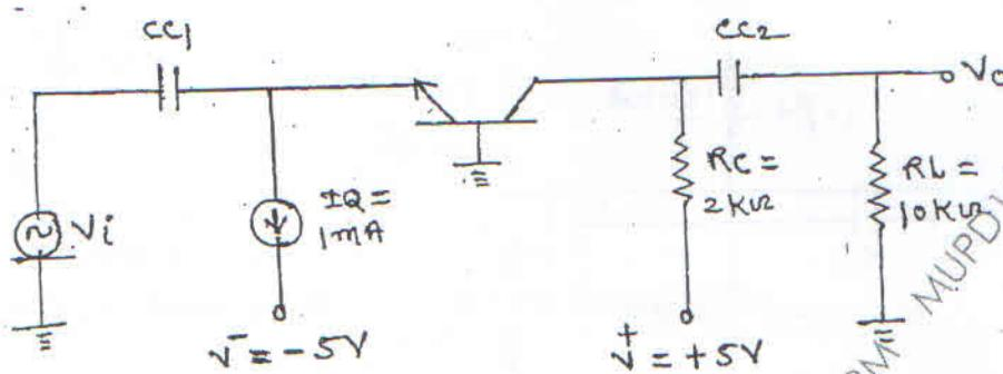
5. (a) For the Amplifier shown determine (i) Q point (ii)  $A_v$ ,  $Z_i$ ,  $Z_o$
